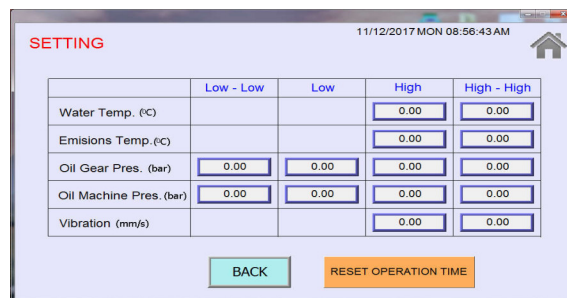
Fig. 4. Control program displaying monitoring parameters
